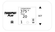
**14.7** Press "dot" button for 3 seconds to switch between each combination settings.
