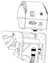
1.2 Fasten the control box onto the machine with 4 screws tightly.
