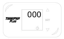
**Note:** If temperature on heat platen is higher than circuit board shows,pls raise the Pb value.
