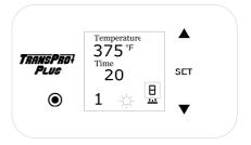
**14.8** Press "set" button and "arrow" button to preset each temperature and time combination setting.
