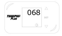
**11.3** Press "set" button to select "ctr" mode, press up and down button to set value at 0 or 1, 0 for celsius, 1 for Fahrenheit
