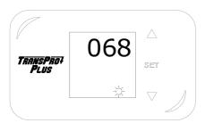
**13.3** Press "set" button to select "Pb" mode. Press up and down button to make temperature calibration.
