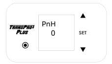
**14.4** Customer can set value from 0~5. For example, if customer set value 3, then in the main screen of the control board, customer can pre-set 3 different temperature and time combinations.
