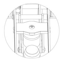
**3.2** Turn the "Ramspin" system into picture position,machine works under manual mode. Once close the machine, electromagnet does not work to hold machine closed. Once time is counting down to 0, machine needs to be opened by hand.
