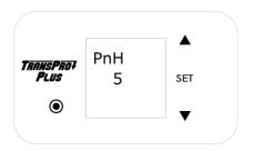
**14.5** For "PnH" value, if customer set value with "0", then in the main screen of control board there is no pre-setting indicator shows at the bottom left corner.
