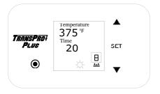
**14.6** If customer set value with 1~4,then in the main screeen of control board there will be indicator shows at the bottom left corner.
